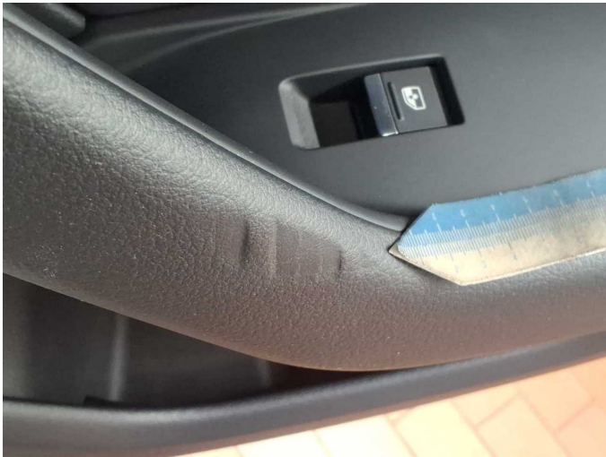
Damage 1: Trim / covers: Door trim - rear right side (Druckstelle Reifen) - Smart repair
