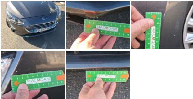
Door RR, Dent(s) and scratch(es), Acceptable
