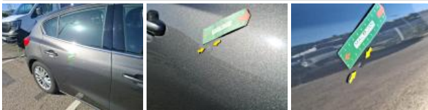
Bumper spoiler Rear, Scratch(es), Repair and paint (complete)
