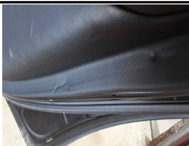
Damage #7: Trim / covers: Door trim - rear right side - Damaged - Replace
