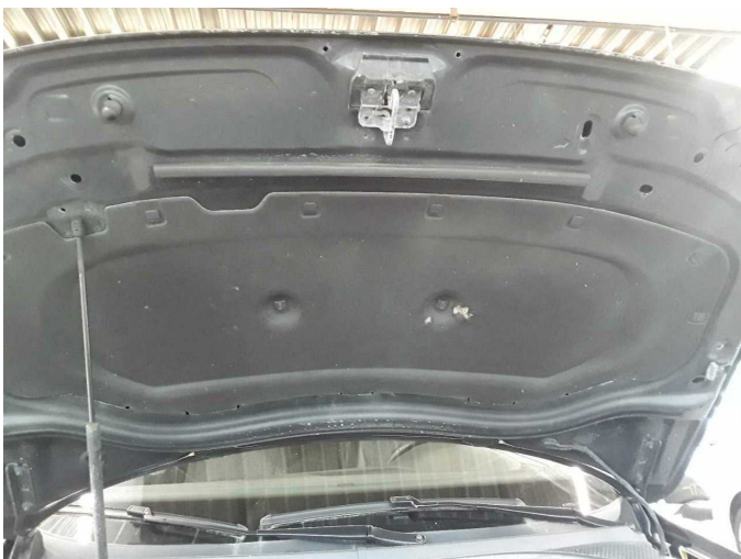
Damage 5: Bonnet: Insulation lining - Damaged - Replace
