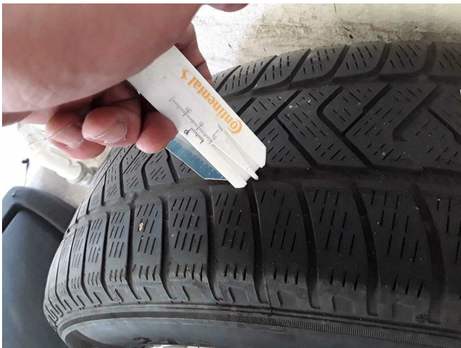
Damage 6: 2nd wheel set: 2 tyres - Does not meet the leasing specifications - Replace
