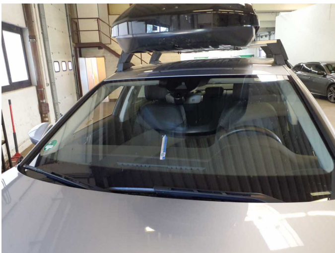
Damage 6: Vehicle glazing: Windscreen - Broken / torn - Replace
