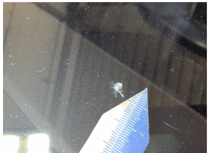
Damage 6: Vehicle glazing: Windscreen - Broken / torn - Replace
