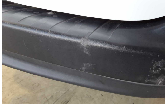
Damage 4: Rear bumper: Rear bumper - Scratch(es) - Loss in value
