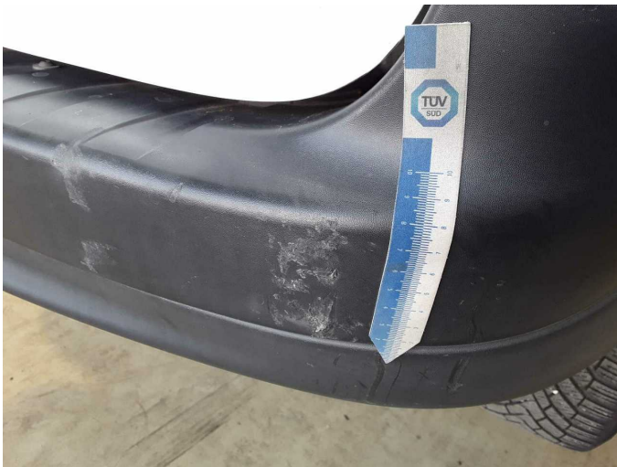
Damage 4: Rear bumper: Rear bumper - Scratch(es) - Loss in value
