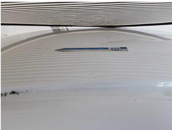
Damage 2: Roof: Roof - dent(s) - Smooth repair work
