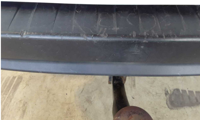
Damage 4: Rear bumper: Rear bumper - Scratch(es) - Loss in value
