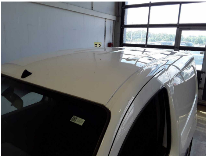
Damage 2: Roof: Roof - dent(s) - Smooth repair work
