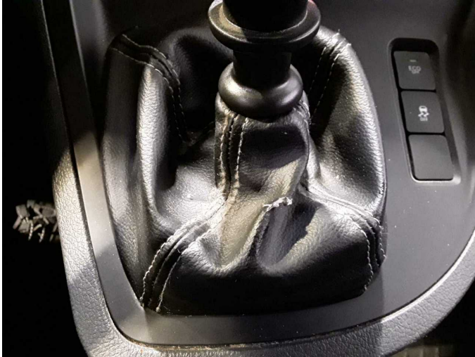
Damage 3: Gearbox: Gear stick collar - Broken / torn - Replace
