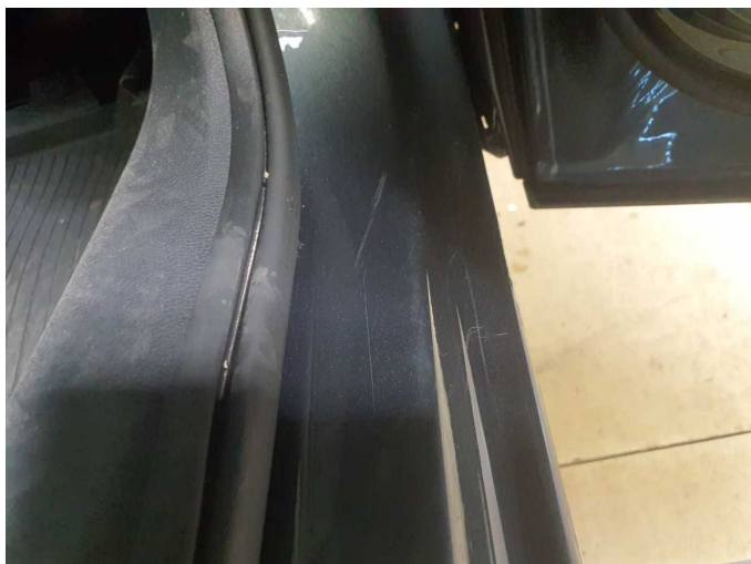
Damage 6: Side panel - rear right side: Sill - Scratch(es) - Smart repair
