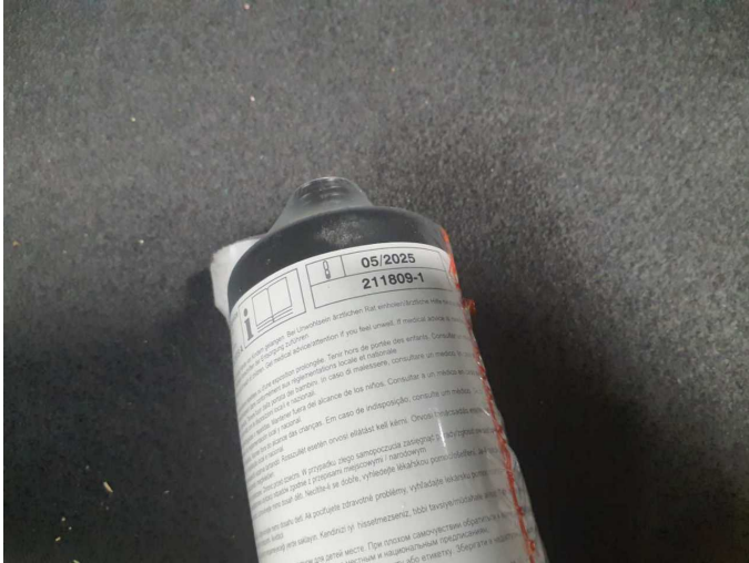
Damage 1: Equipment: Tirefit filler - Expired - Replace
