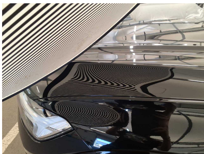
Damage 9: Bonnet: Bonnet - Dent / paintcoat damage - Paint
