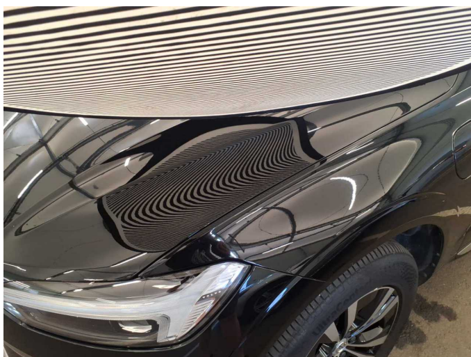
Damage 9: Bonnet: Bonnet - Dent / paintcoat damage - Paint
