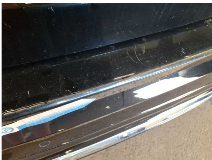
Damage 6: Rear bumper: Rear bumper - Scratch(es) - Paint
