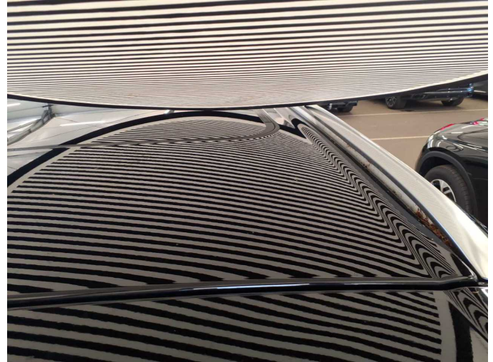
Damage 10: Roof: Roof - Dent / paintcoat damage - Paint
