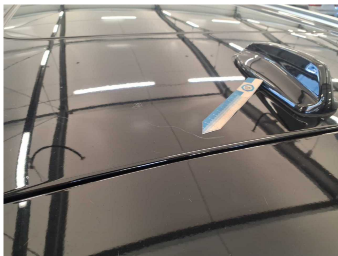
Damage 10: Roof: Roof - Dent / paintcoat damage - Paint
