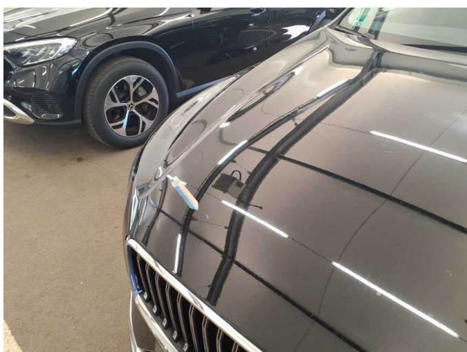
Damage 9: Bonnet: Bonnet - Dent / paintcoat damage - Paint
