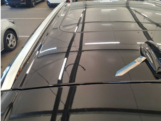
Damage 10: Roof: Roof - Dent / paintcoat damage - Paint
