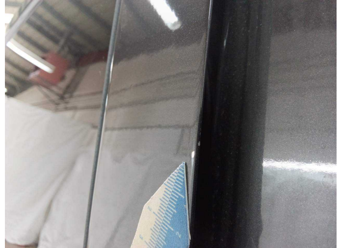
Damage 2: Door - rear right side: Door edge - Scratch(es) - Smart repair
