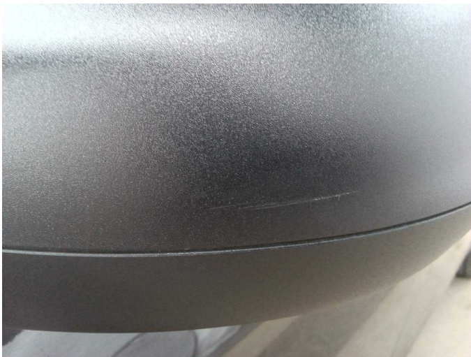
Wear and tear 7: Wing mirror - left side: Cap - Scratch(es) - No deduction
