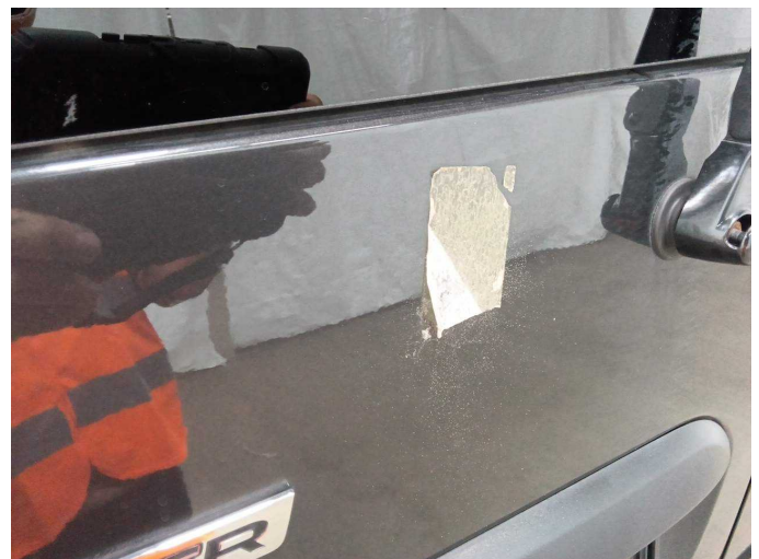
Damage 3: Body: Body - Glued / labelled - De-glug / neutralise
