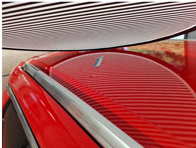
Damage 3: Roof: Roof - dent(s) - Smooth repair work
