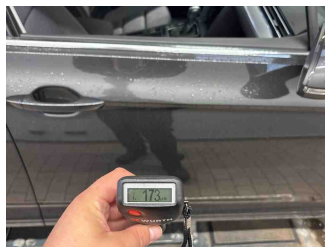
Paint thickness Door FR
