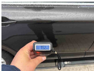
Paint thickness Door RR
