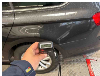
Paint thickness Wing RL
