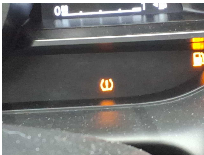
Damage 2: Instrument panel: Indicator light (Reifendruckkontrollsystem) - on - Perform diagnosis
