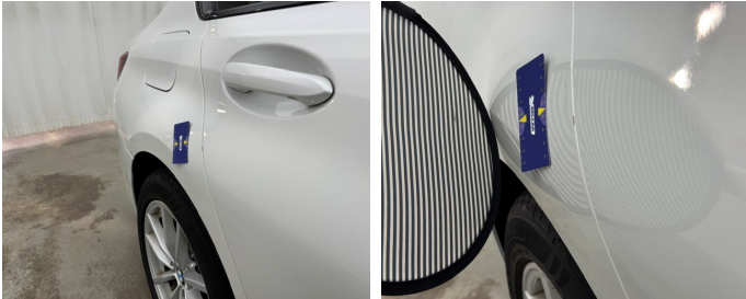
Wing Rear Right // Repair & Painting-scratch + dent
