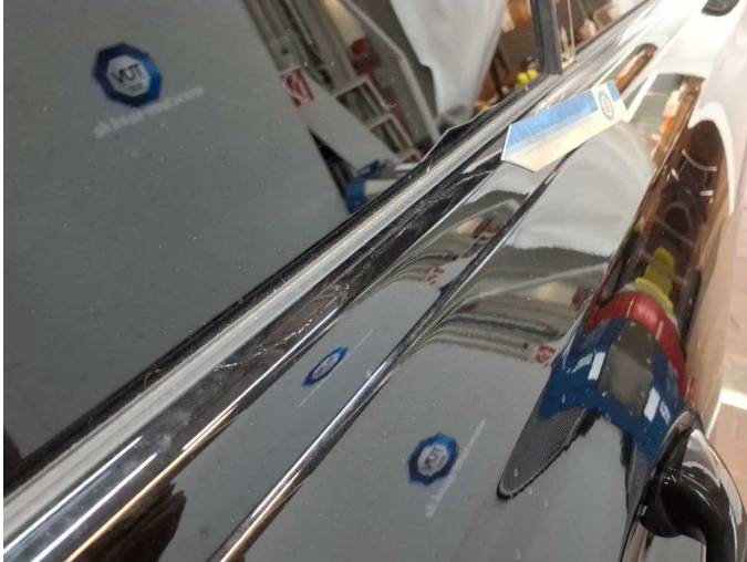
Damage 6: Door - front right side: Brightware - upper - Scratch(es) - Smart repair
