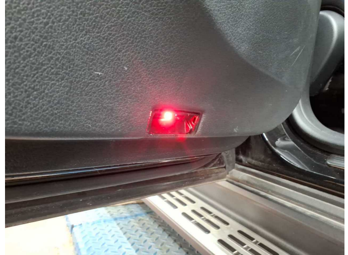
Damage 1: Trim / covers: Door trim - rear left side (Lichtabdeckung) - Missing - Replace
