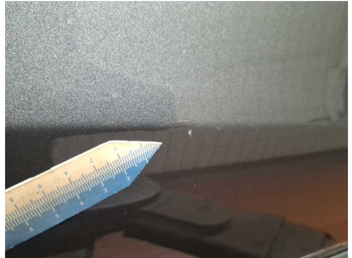
Damage 2: Door - front right side: Door - Stone chips - Smart repair
