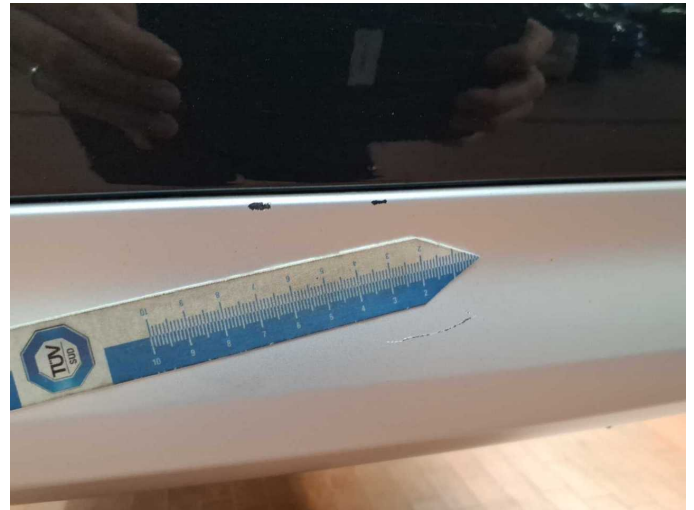
Damage 3: Rear bumper: Spoiler - Scratched - Replace
