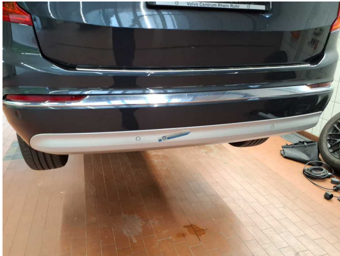
Damage 3: Rear bumper: Spoiler - Scratched - Replace
