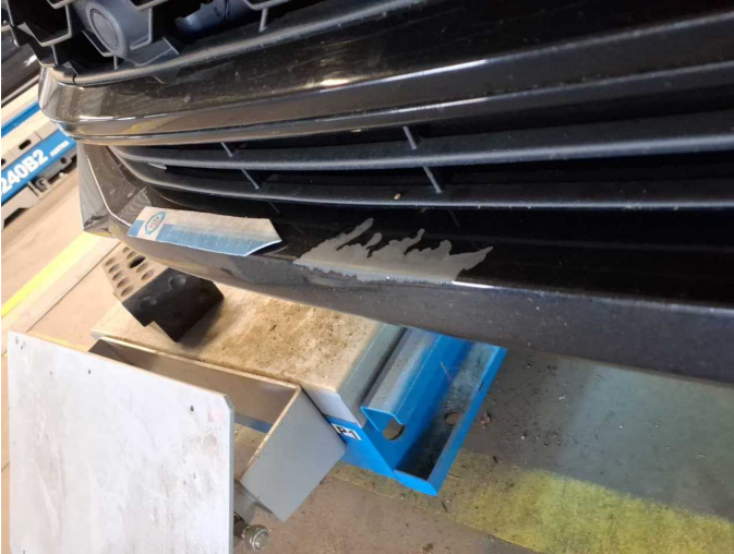
Damage 3: Front bumper: Spoiler - Paint defect - Paint
