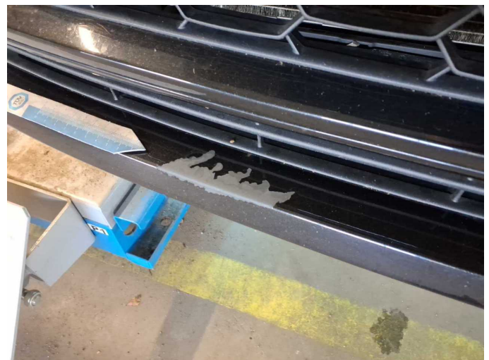
Damage 3: Front bumper: Spoiler - Paint defect - Paint
