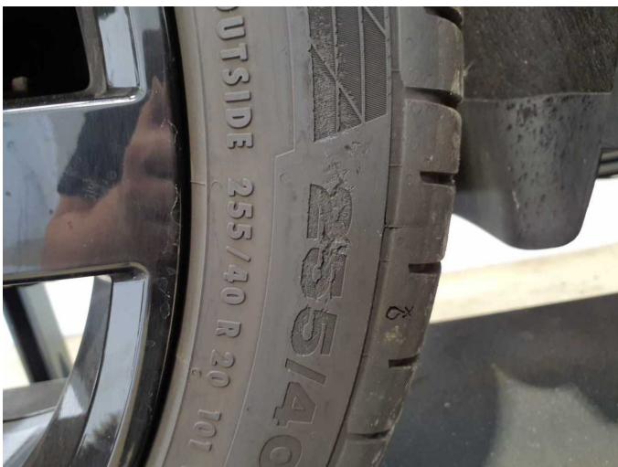
Damage 5: Wheel / tyres: Tyre - rear right side - Scratch(es) - Replace
