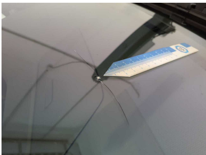
Damage 10: Vehicle glazing: Windscreen - Broken / torn - Replace
