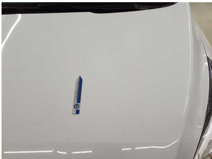
Damage 3: Bonnet: Bonnet - Stone chips - Paint
