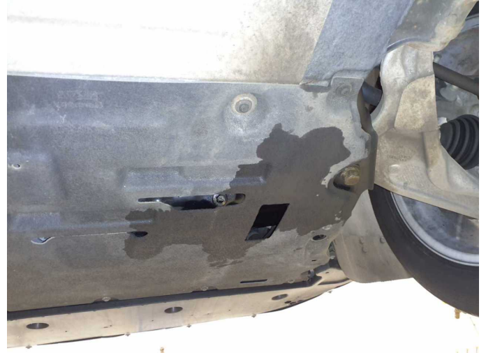
Damage 1: Engine: Engine - Leaking - Perform diagnosis
