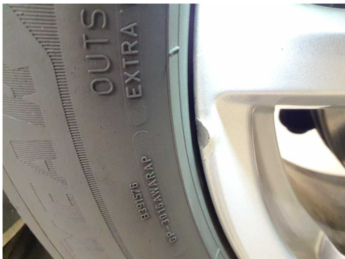
Damage 2: Wheel / tyres: Alloy rim - front right side (Materialabtrag) - Damaged - Replace
