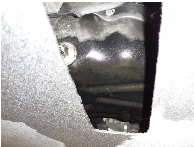
Damage 1: Engine: Engine - Leaking - Perform diagnosis
