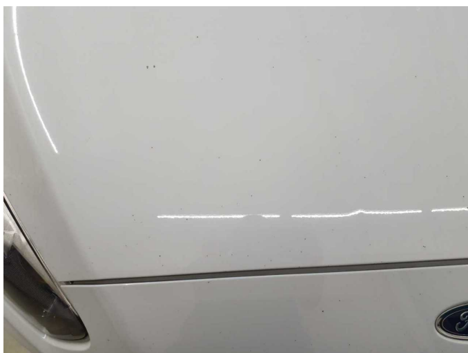
Damage 3: Bonnet: Bonnet - Stone chips - Paint
