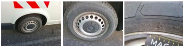
Tyre RL, Out of tolerance, Replace
