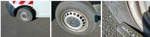
Side wall RL, Dent(s), Repair and paint (complete)
