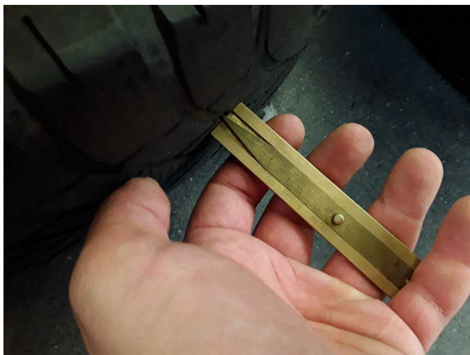
Damage 2: 2nd wheel set: Tyres - complete set (215,65,17 w.) - Worn - Replace
