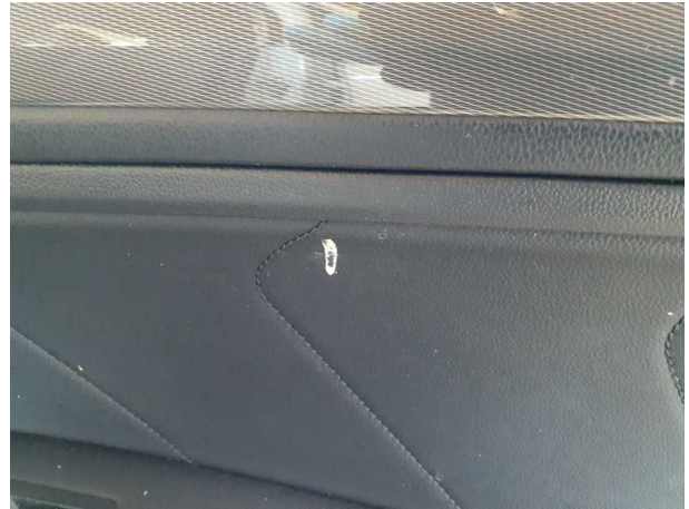
Damage #1: Trim / covers: Door trim - front right side - Soiled - Conditioning
