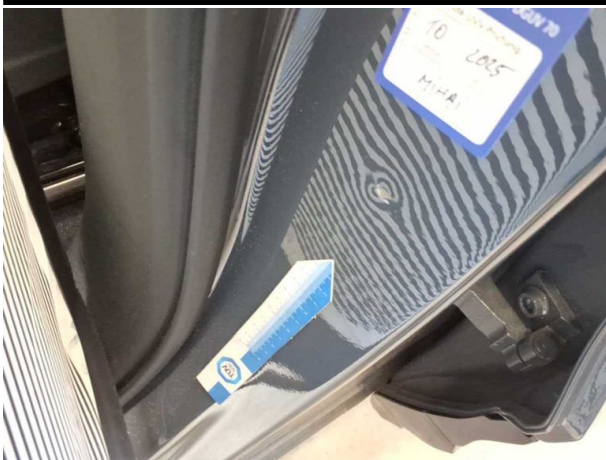
Damage #3: Body: B-pillar - left side - Dent / paintcoat damage - Smart repair
