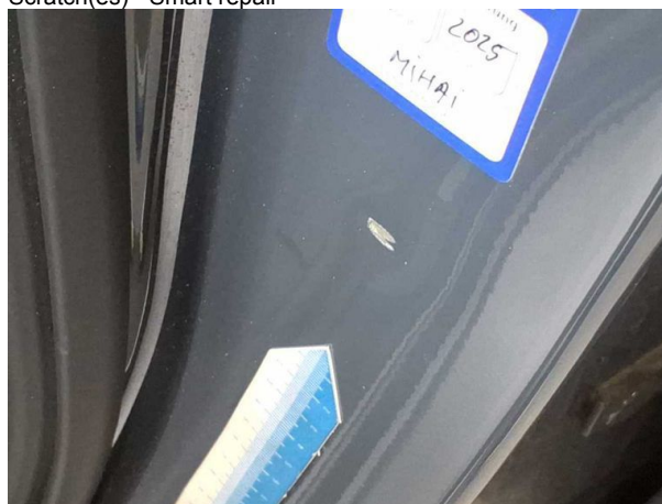
Damage #3: Body: B-pillar - left side - Dent / paintcoat damage - Smart repair
