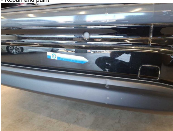
Damage #7: Rear bumper: Bumper with Parktronic - Dent / paintcoat damage - Repair and paint
