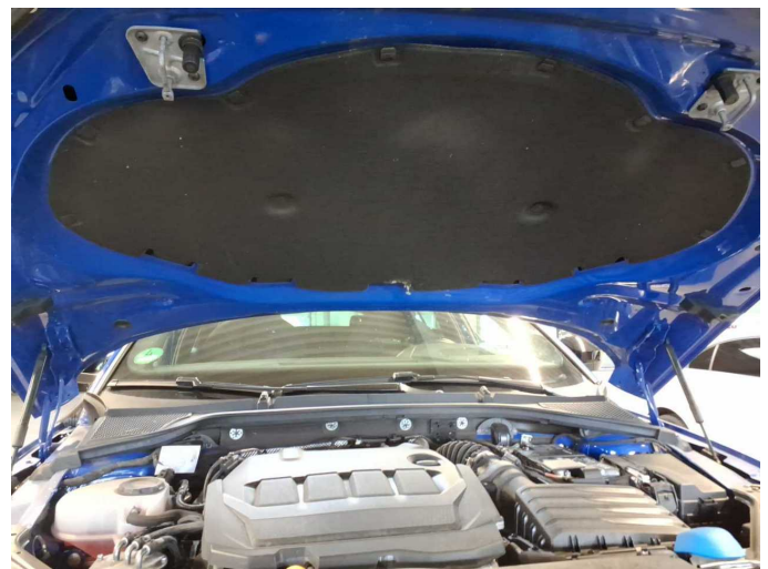
Damage 2: Bonnet: Insulation lining - Damage caused by marten / rodent - Replace
