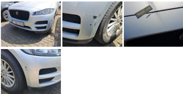
Wing FL, Scratch(es), Repair and paint (complete)
