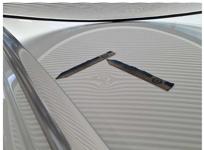
Damage 5: Roof: Roof - dent(s) - Smooth repair work
