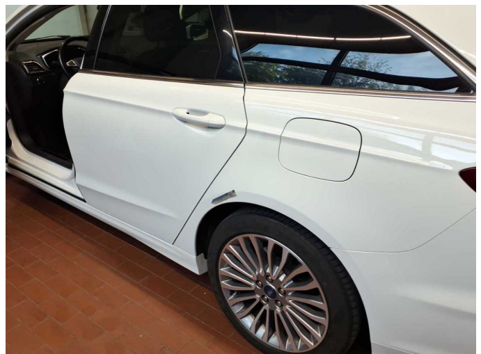
Damage 3: Side panel - rear left side: Elbow - dent(s) - Smart repair
