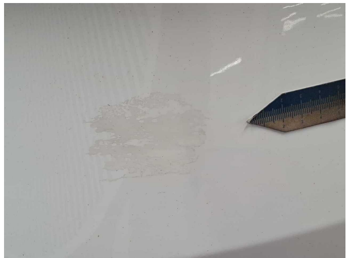
Damage 2: Boot lid / rear door: Boot lid (Klebereste) - Glued / labelled - De-glu / neutralise
