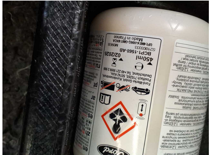
Damage 1: Equipment: Tirefit filler - Expired - Replace
