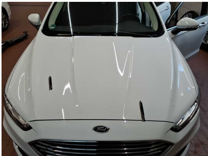
Damage 9: Bonnet: Bonnet - Stone chips - Paint
