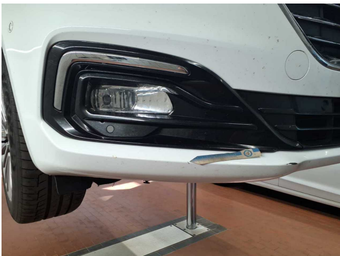
Damage 8: Front bumper: Front bumper - Scratched - Paint
