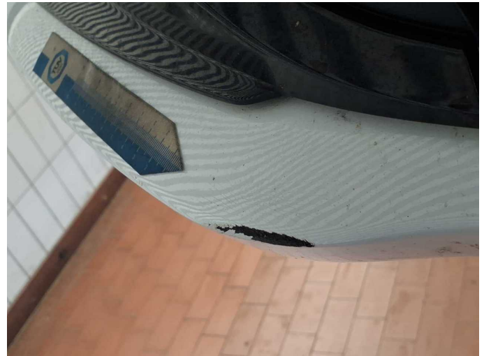
Damage 8: Front bumper: Front bumper - Scratched - Paint
