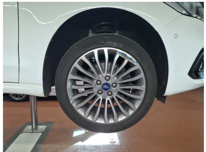
Damage 7: Wheel / tyres: Alloy rim - front right side - Scratched - Replace
