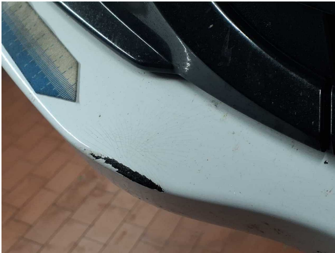
Damage 8: Front bumper: Front bumper - Scratched - Paint
