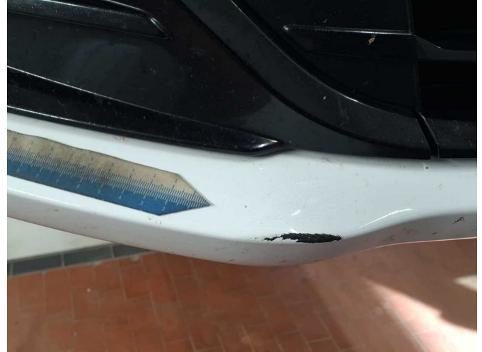
Damage 8: Front bumper: Front bumper - Scratched - Paint
