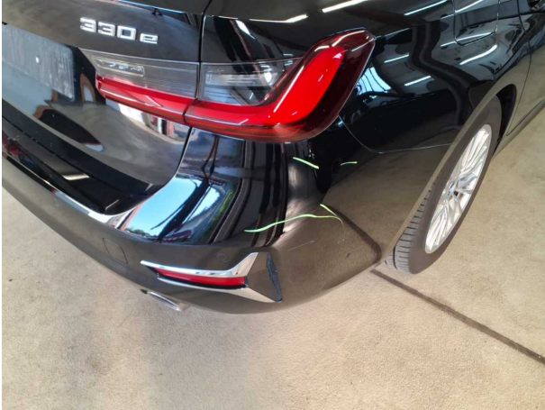
Damage #1: Rear bumper: Rear bumper - Scratched - Repair and paint
