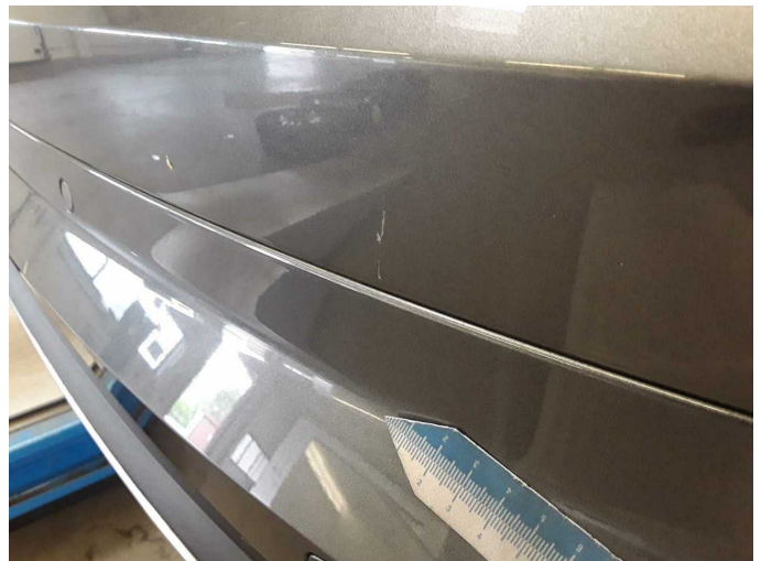
Damage 4: Rear bumper: Rear bumper - Scratch(es) - Smart repair
