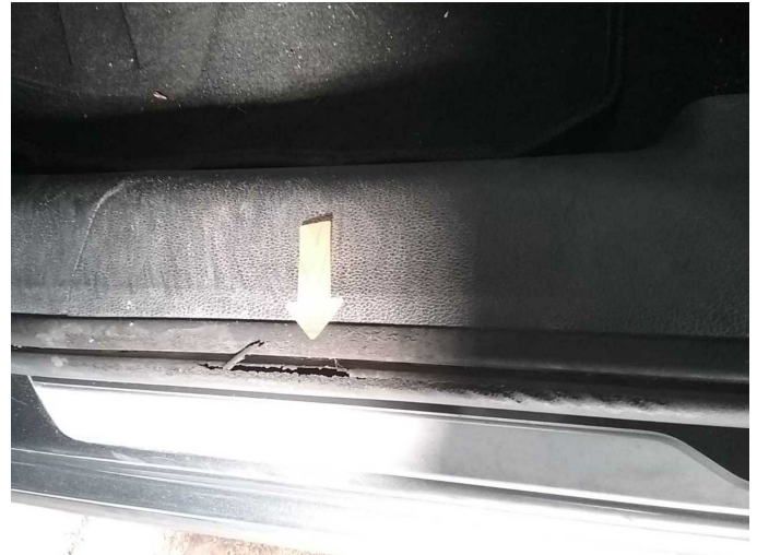
Damage 5: Body: Door seal - front left side - Broken / torn - Replace
