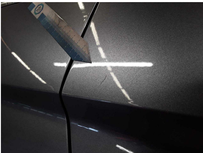
Damage 6: Door - rear right side: Door - Dent / paintcoat damage - Smart repair
