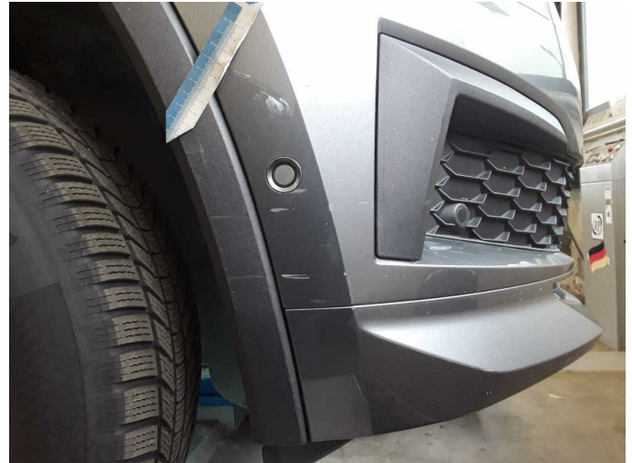
Damage 7: Mudguard - right side: Wheel arch - Scratched - Replace
