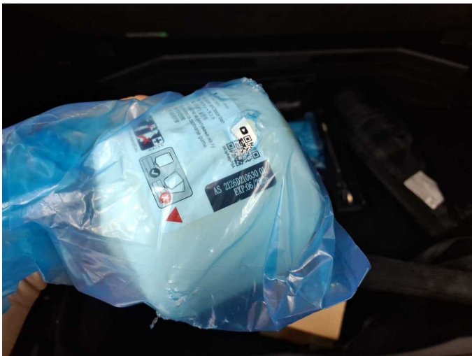
Damage 2: Equipment: Tirefit filler - Expired - Replace
