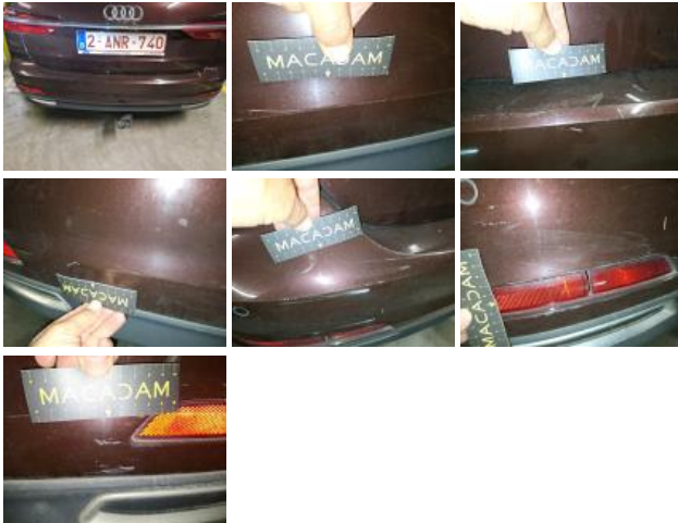
Bumper moulding R, Scratch(es), Replace
