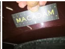
Outside rear-view mirror housing L, Scratch(es), Acceptable
