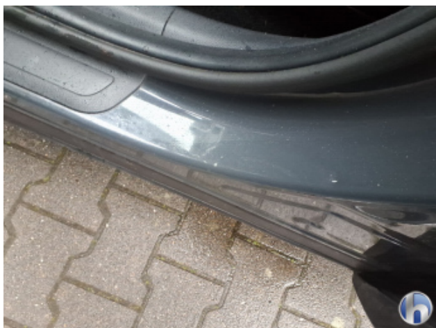
2. Schweller - Links Kratzer - Smart Repair
