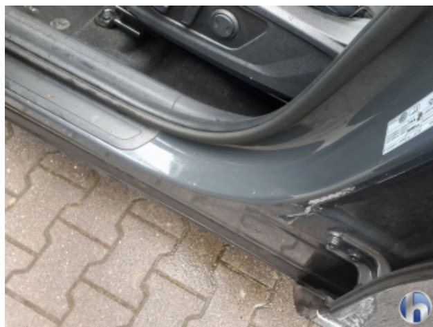
2. Schweller - Links Kratzer - Smart Repair
