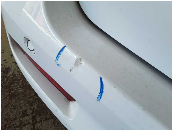
Damage #7: Rear bumper: Rear bumper - Deformed - Replace
