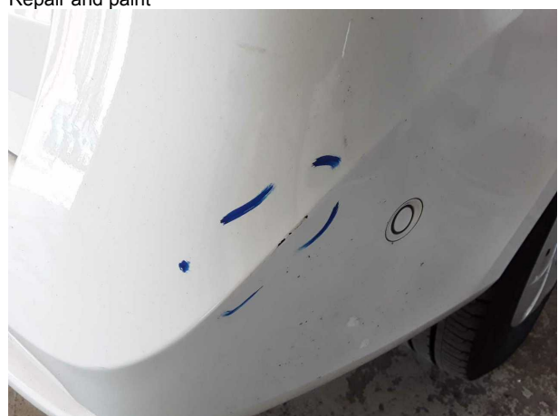
Damage #7: Rear bumper: Rear bumper - Deformed - Replace
