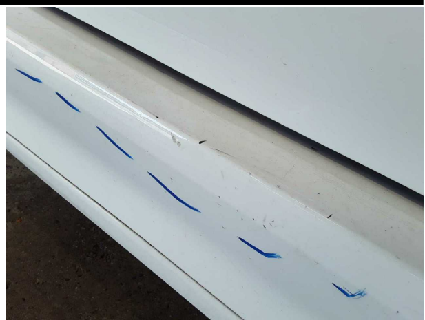
Damage #7: Rear bumper: Rear bumper - Deformed - Replace
