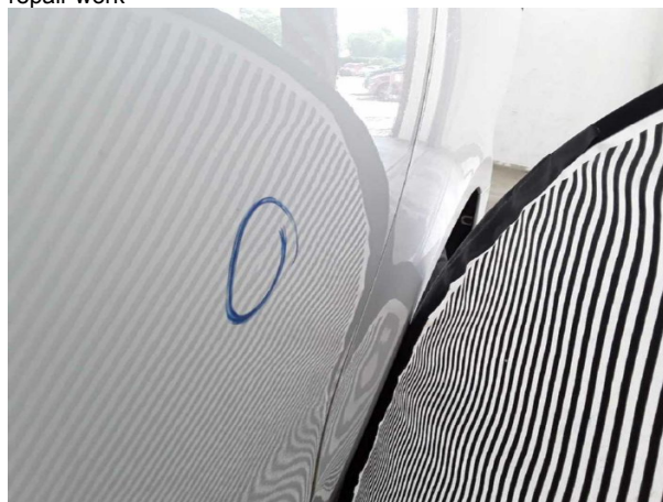
Damage #3: Sliding door - left side: Sliding door with glass panel - dent(s) - Smooth repair work
