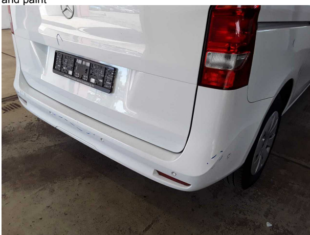
Damage #7: Rear bumper: Rear bumper - Deformed - Replace
