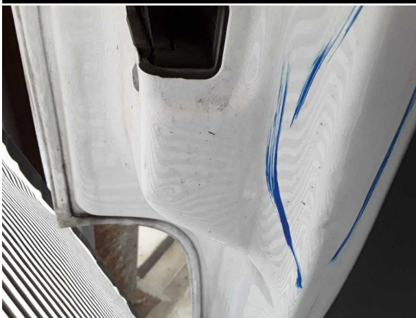
Damage #8: Door - front left side: Door - Dent / paintcoat damage - Repair and paint
