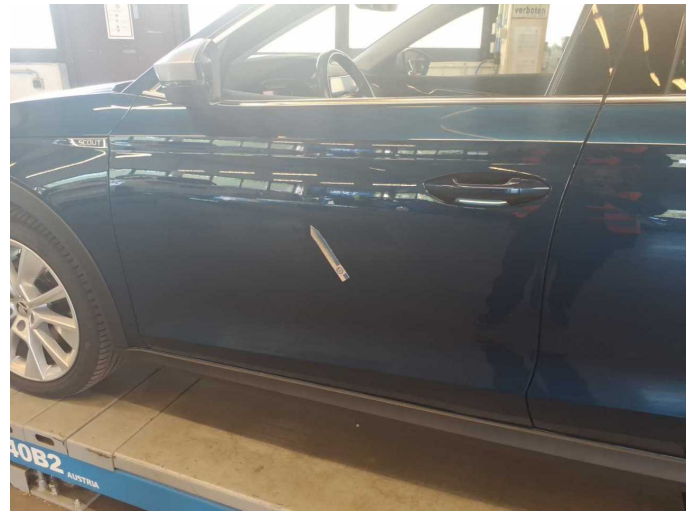
Damage 7: Door - front left side: Door - Scratched - Paint
