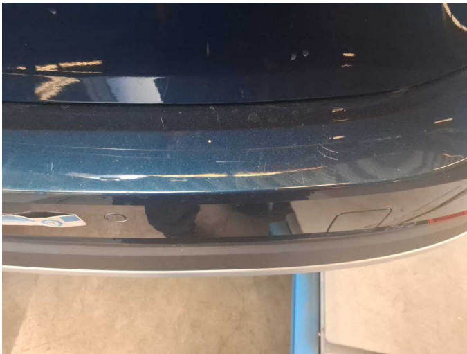
Damage 6: Rear bumper: Rear bumper - Scratched - Paint
