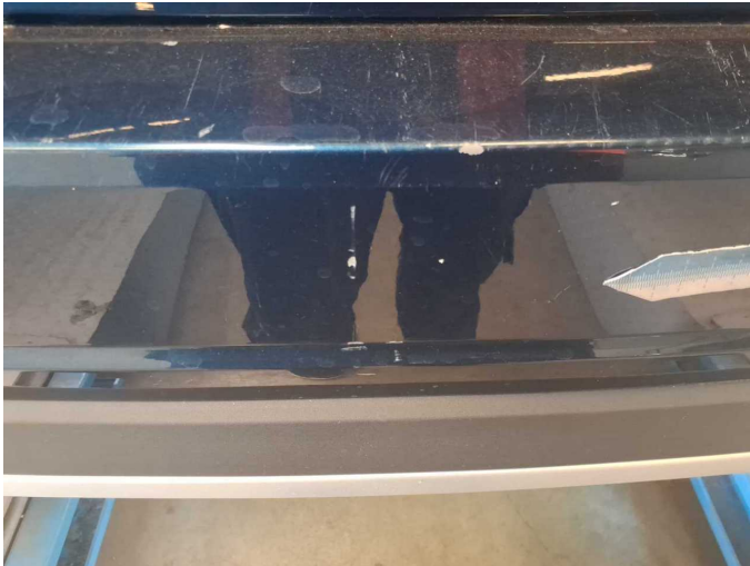
Damage 6: Rear bumper: Rear bumper - Scratched - Paint
