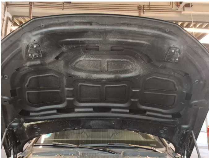
Damage 4: Bonnet: Insulation lining - Missing - Replace
