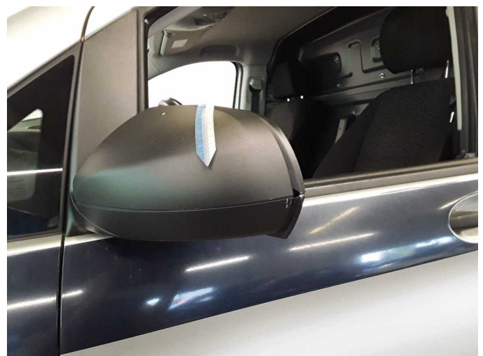
Damage 7: Wing mirror - left side: Mirror housing - Broken / torn - Replace
