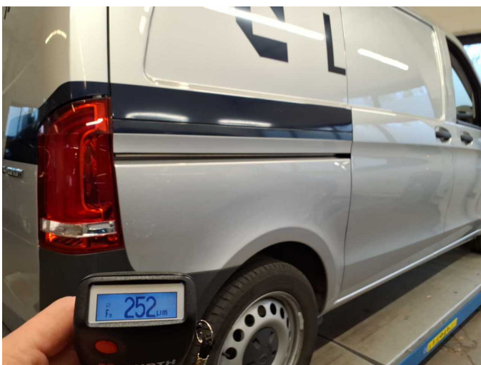
Repainting 1: Side panel - rear right side
