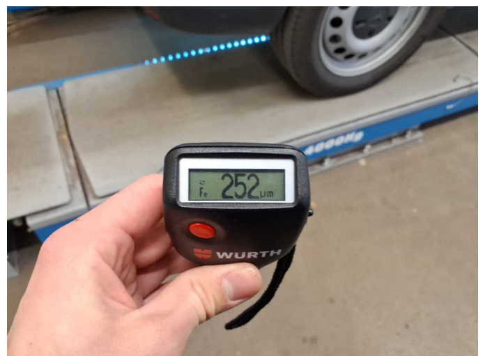
Repainting 1: Side panel - rear right side
