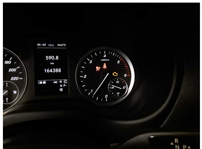
Damage 3: Airbag systems: Airbag - front left side (und Motorkontrolle leuchtet, nicht fahrbereit) - Functional / admissibility - Perform diagnosis
