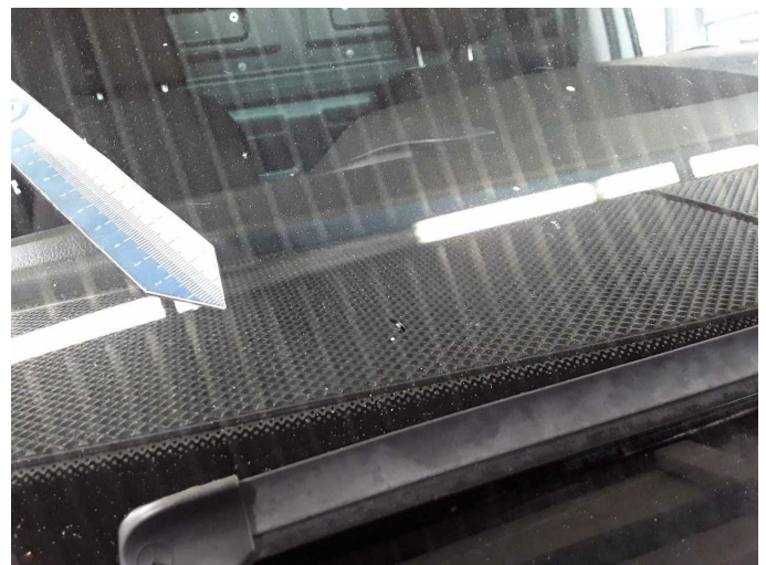
Wear and tear 5: Vehicle glazing: Windscreen (Rissbildung) - Stone chips - No deduction
