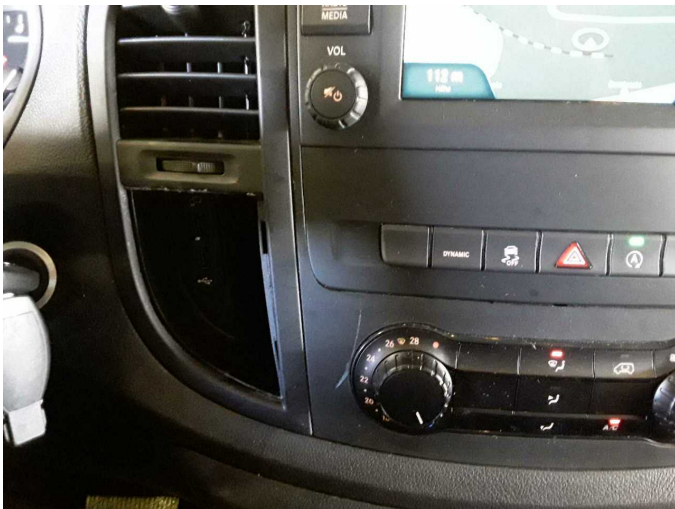
Damage 2: Instrument panel: Stowage compartment - Broken / torn - Replace
