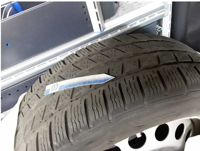
Damage 4: 2nd wheel set: 2 tyres - Does not meet the leasing specifications - Replace
