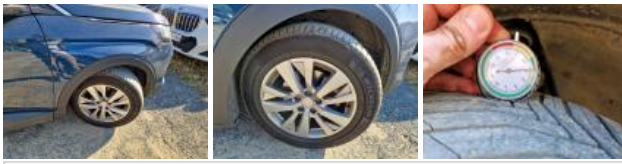
Tyre FL, Out of tolerance, Replace
