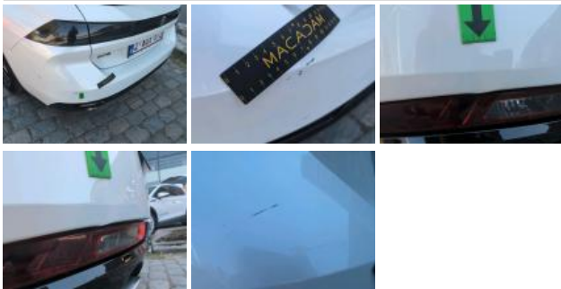
Fog light RR, Crack, Replace
