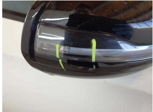
Damage #1: Indicator - front: Mirror - right side - Scratched - Replace
