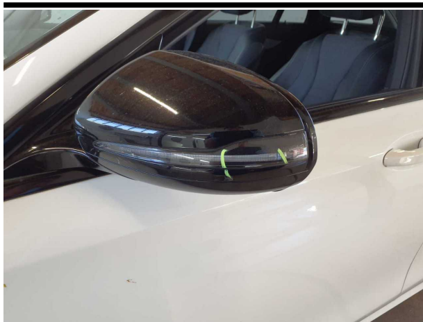
Damage #4: Indicator - front: Mirror - left side - Scratched - Replace
