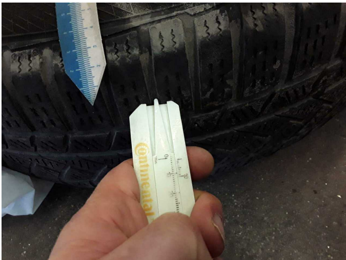
Damage 1: 2nd wheel set: 2 tyres - Worn - Replace
