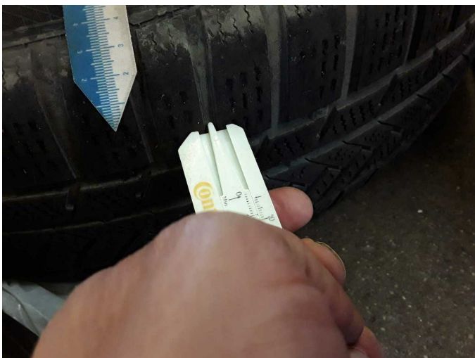
Damage 1: 2nd wheel set: 2 tyres - Worn - Replace
