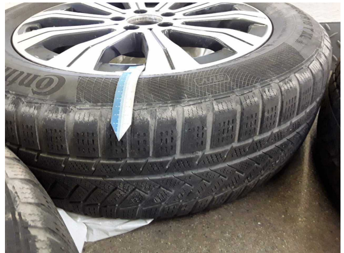
Damage 1: 2nd wheel set: 2 tyres - Worn - Replace
