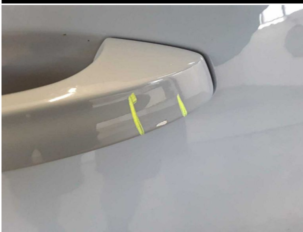
Damage #6: Door - front right side: Door handle - outside - Scratched - Smart repair
