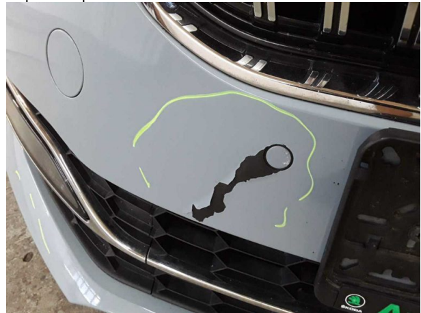
Damage #7: Front bumper: Front bumper - Paint defect - Repair and paint
