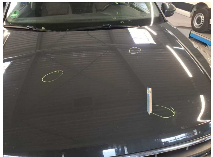
Damage 8: Bonnet: Bonnet - dent(s) - Smooth repair work
