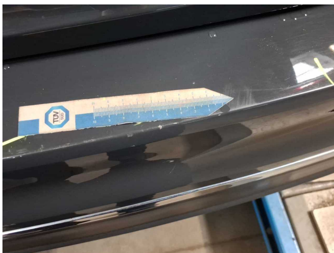
Damage 12: Rear bumper: Rear bumper - Scratch(es) - Paint
