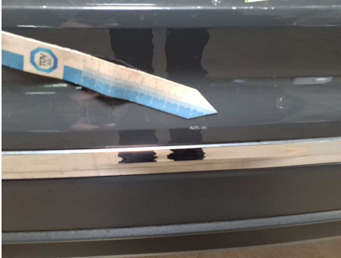
Damage 12: Rear bumper: Rear bumper - Scratch(es) - Paint
