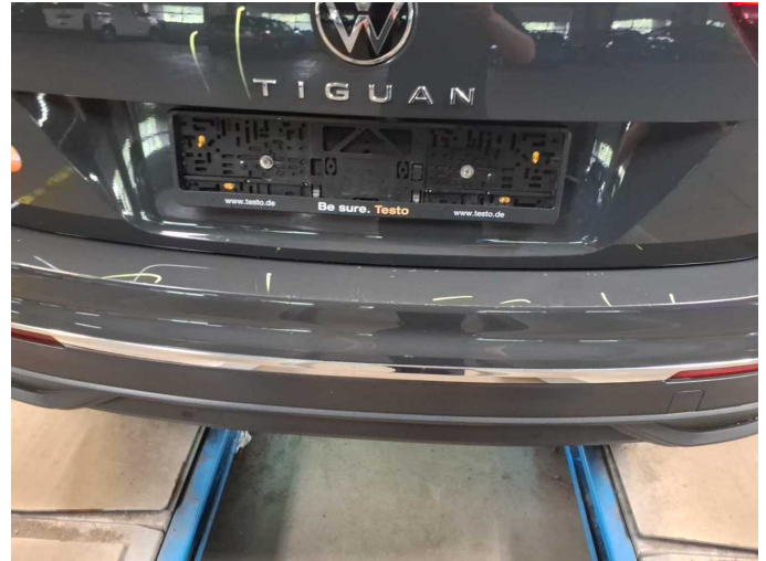
Damage 12: Rear bumper: Rear bumper - Scratch(es) - Paint
