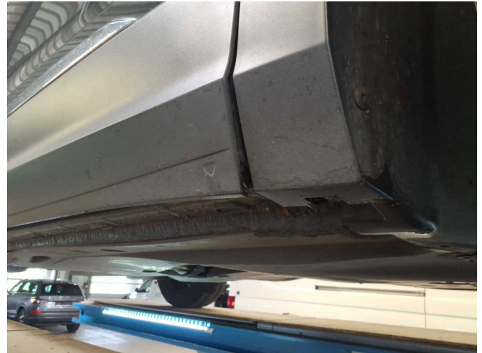
Damage 4: Door - front right side: Brightware - lower - Malposition - Un- / install
