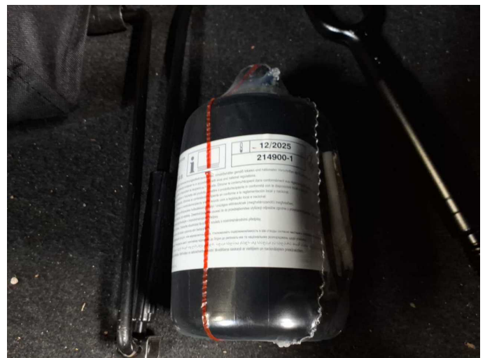
Damage 3: Equipment: Tirefit filler - Expired - Replace
