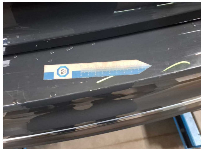
Damage 12: Rear bumper: Rear bumper - Scratch(es) - Paint
