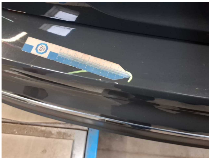
Damage 12: Rear bumper: Rear bumper - Scratch(es) - Paint
