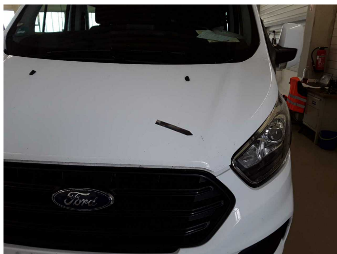
Damage 10: Bonnet: Bonnet (Steinschläge) - Scratch(es) - Paint
