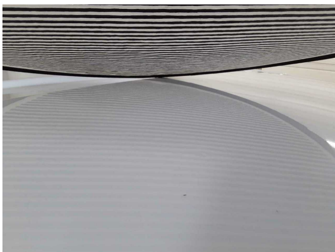
Damage 7: Roof: Roof - dent(s) - Smart repair
