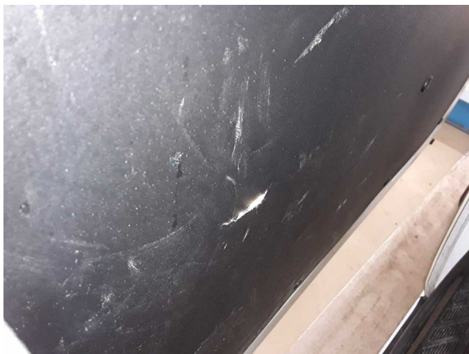
Damage 8: Sliding door, right: Trim washable - lower - Broken / torn - Replace
