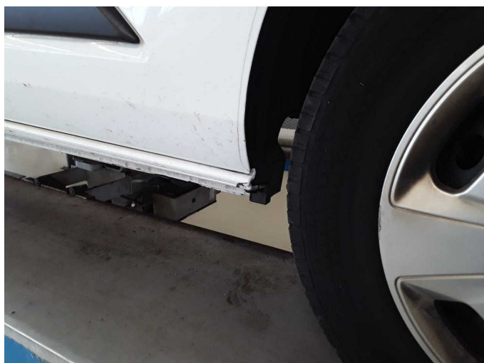
Damage 5: Mudguard - right side: Mud flap - Missing - Replace
