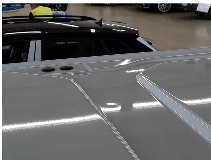
Damage 7: Roof: Roof - dent(s) - Smart repair
