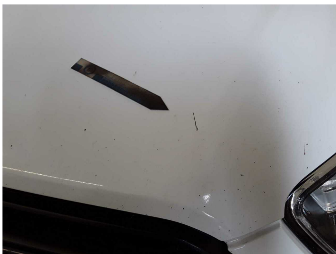
Damage 10: Bonnet: Bonnet (Steinschläge) - Scratch(es) - Paint
