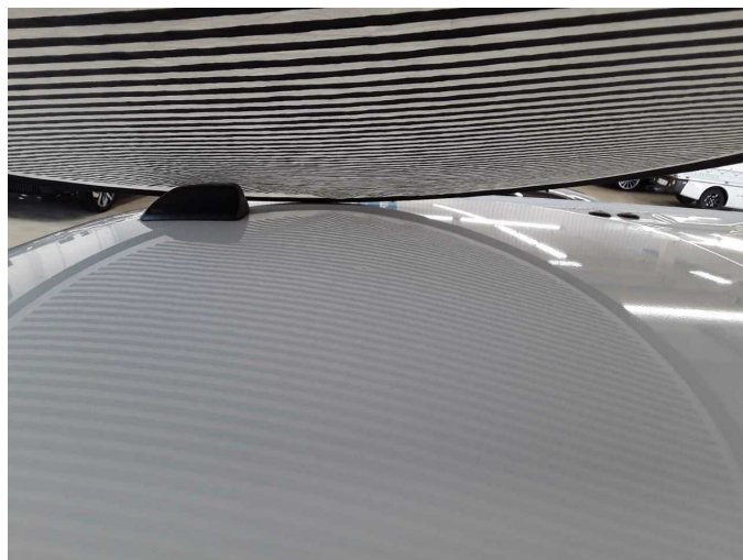
Damage 7: Roof: Roof - dent(s) - Smart repair
