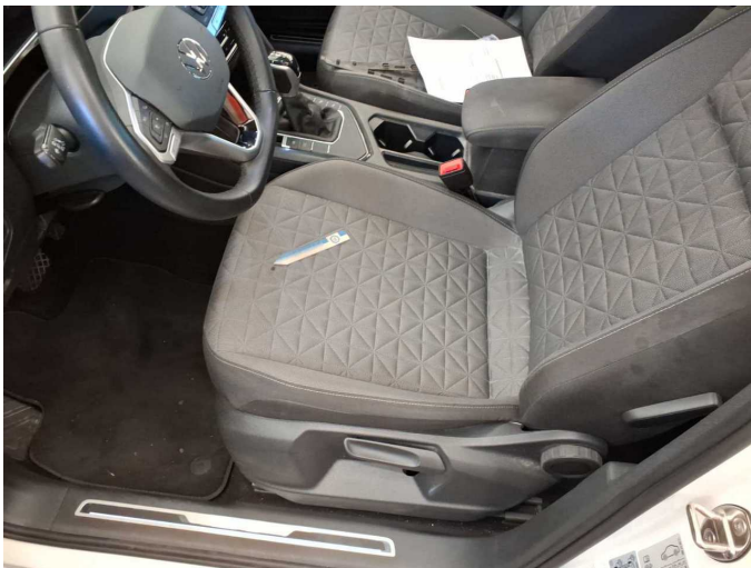
Damage 2: Seat - front: Seat cover - left side - Burn hole (cigarettes) - Replace
