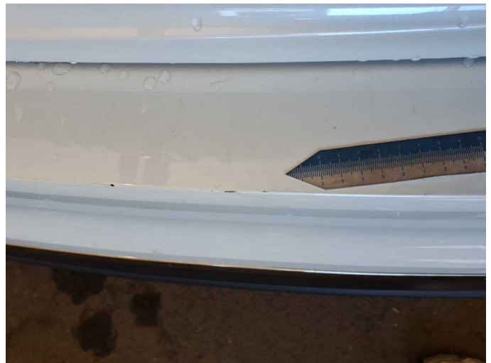
Damage 3: Rear bumper: Rear bumper - Scratch(es) - Paint
