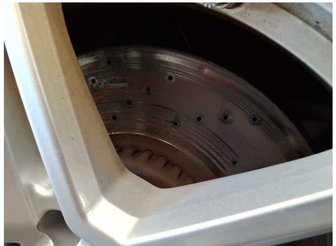
Damage 8: Braking system: Brake discs and brake pads - front (Tragbild mangelhaft, Rost) - Corrosion - Replace
