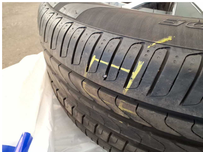
Damage 3: 2nd wheel set: 1 tyre (Fremdkörper in Lauffläche) - Damaged - Replace
