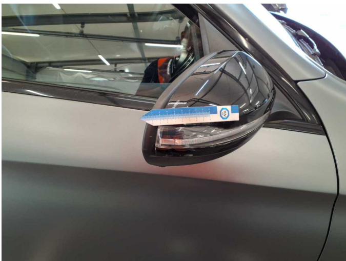
Damage 2: Indicator - front: Mirror - right side - Scratched - Replace
