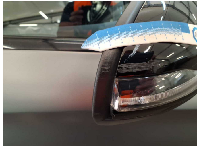
Damage 1: Wing mirror - right side: Mirror housing - Scratched - Smart repair
