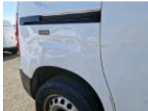
Side wall RR, Dent(s) and scratch(es), Repair and paint (complete)
