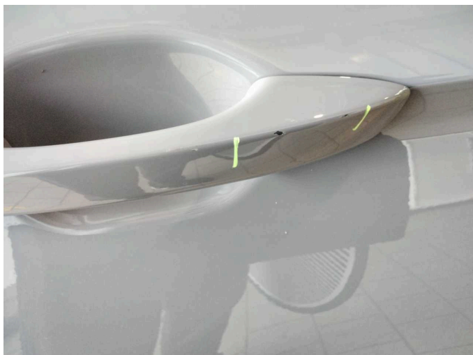
Damage 4: Door - rear right side: Door handle - outside - Scratch(es) - Paint
