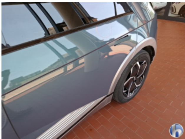
1. Tür Hinten - Links 1 Delle - Sanft Instandsetzen
