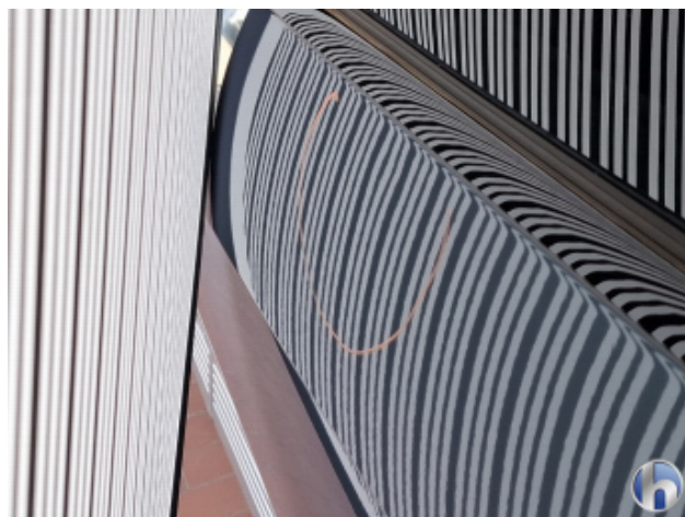
1. Tür Hinten - Links 1 Delle - Sanft Instandsetzen
