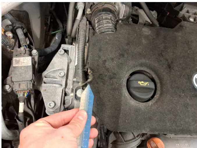
Wear and tear 1: Engine: Engine cover - Broken / torn - No deduction
