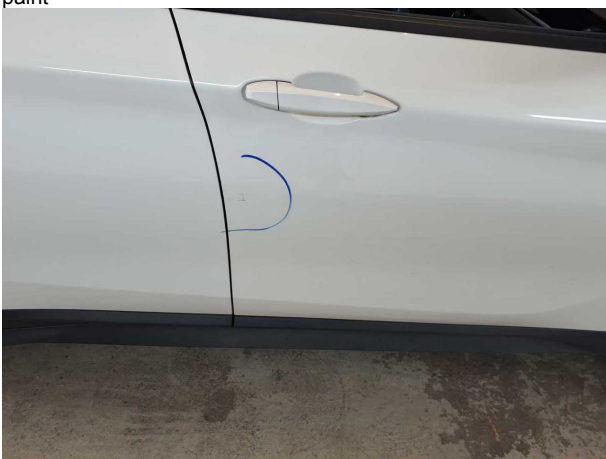
Damage #10: Door - front right side: Door - Scratched - Repair and paint
