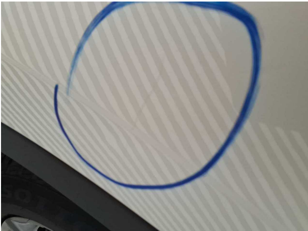
Damage #2: Side panel - rear right side: Side panel - Dent / paintcoat damage - Smart repair
