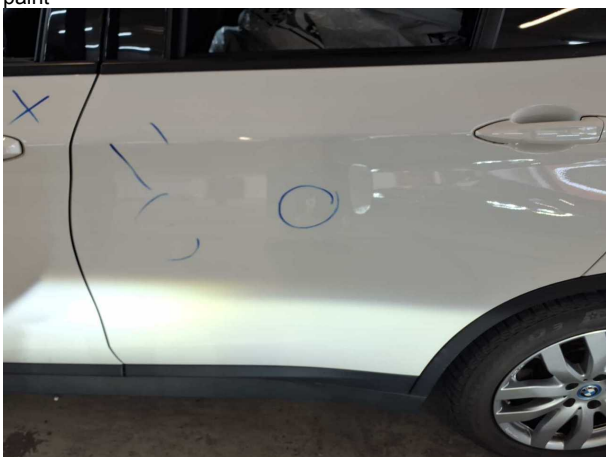
Damage #8: Door - rear left side: Door - Dent / paintcoat damage - Repair and paint
