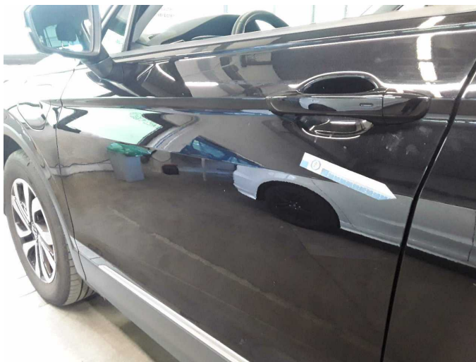
Damage 1: Door - front left side: Door - Scratch(es) - Smart repair
