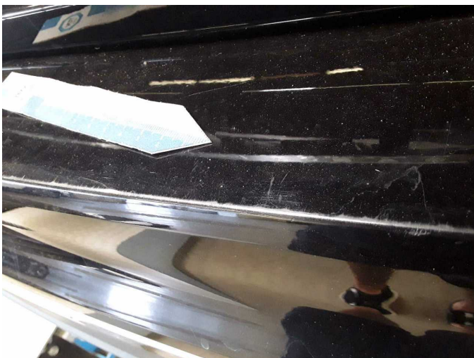
Wear and tear 2: Rear bumper: Rear bumper (Feine Kratzer) - Scratch(es) - No deduction
