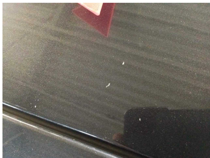
Damage 5: Bonnet: Bonnet - Stone chips - Paint
