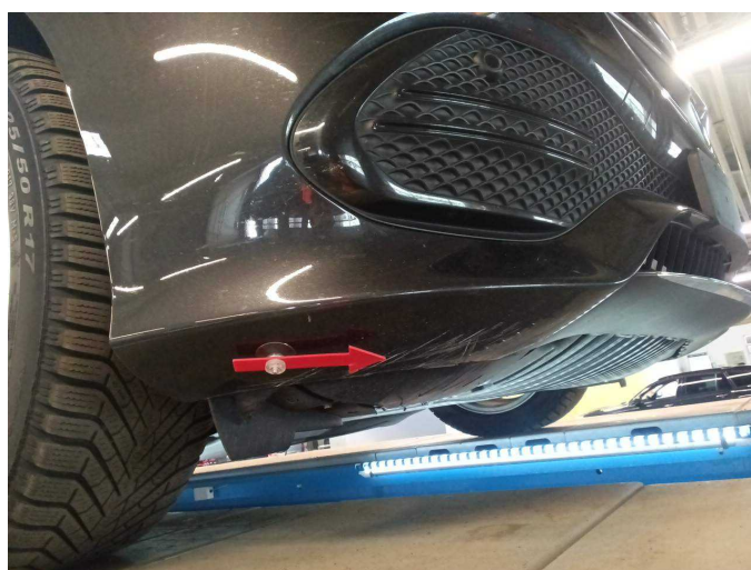
Damage 4: Front bumper: Front bumper - Scratched - Paint
