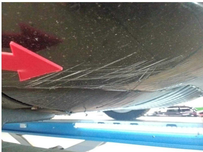
Damage 4: Front bumper: Front bumper - Scratched - Paint
