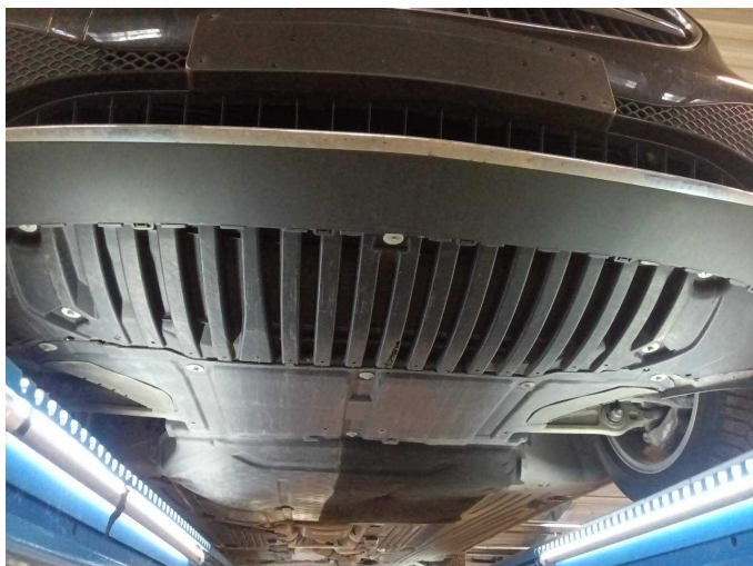
Damage 2: Body: Underbody panelling - Scratched - Replace
