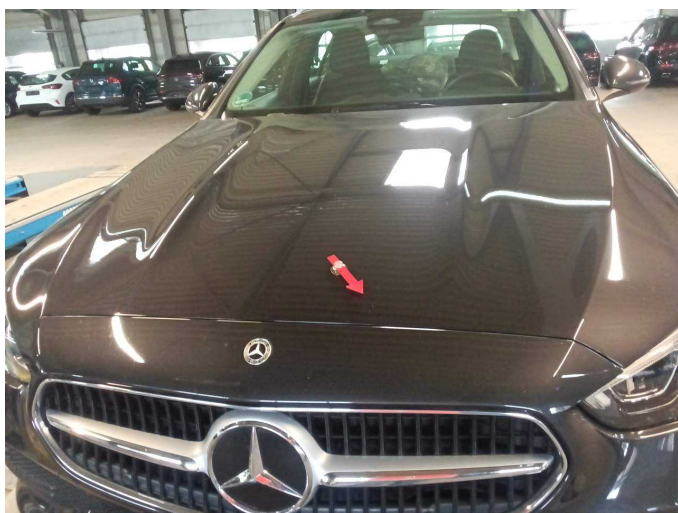
Damage 5: Bonnet: Bonnet - Stone chips - Paint
