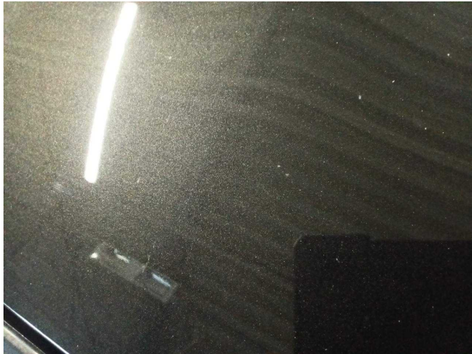
Damage 5: Bonnet: Bonnet - Stone chips - Paint
