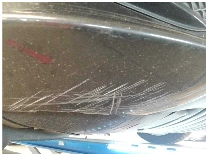
Damage 4: Front bumper: Front bumper - Scratched - Paint
